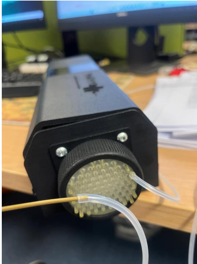
Figure 15: Brass tube coupled to a hose in the pressure Sensor.
